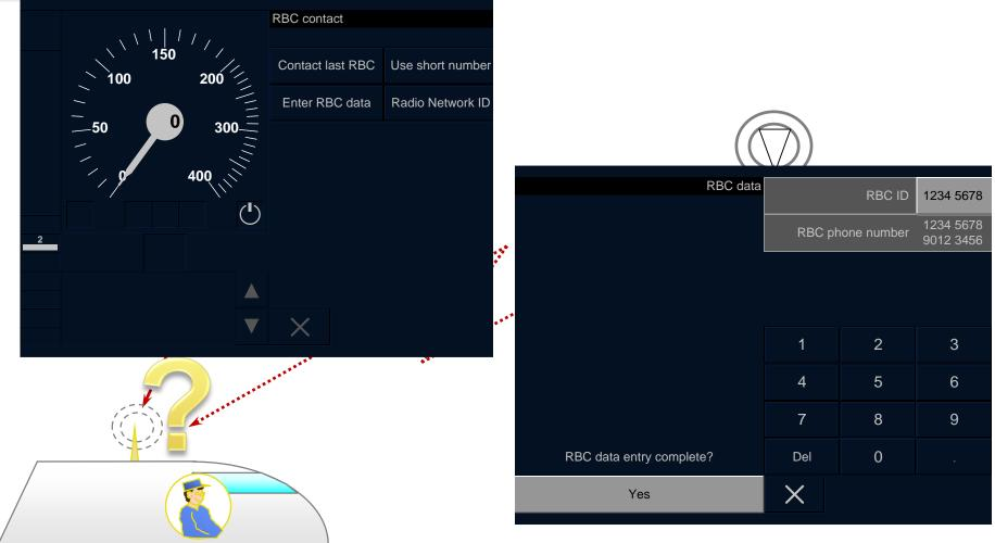
SoM with an invalid position: driver has to validate/enter the RBC train data. How does the driver know which RBC data is required? Especially near a RBC-RBC HO location. Note: RBC data errors take (from experience) a long time to (detect and) resolve.
