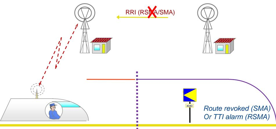
ACC RBC shortens MA on RRI does HO RBC use a RSMA or SMA (SS039 4.5.1.2) For a revoked signal the MA is always shortened (SMA). The cooperative revocation is used to release the route. For a TTI alarm only a cooperative revocation (RSMA) is used to allow the train to continue if it can not stop in time. How can the difference be made across the RBC-RBC interface?
