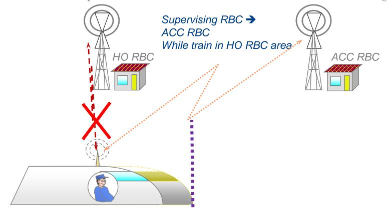
Balise or communication error; CR1228: SB stop in HO RBC area. EoA at front of the train. Max-safe in ACC RBC area. ACC RBC supervising. ACC RBC can not give MA track description for HO RBC area. How is the MA extension possible? How to continue?
