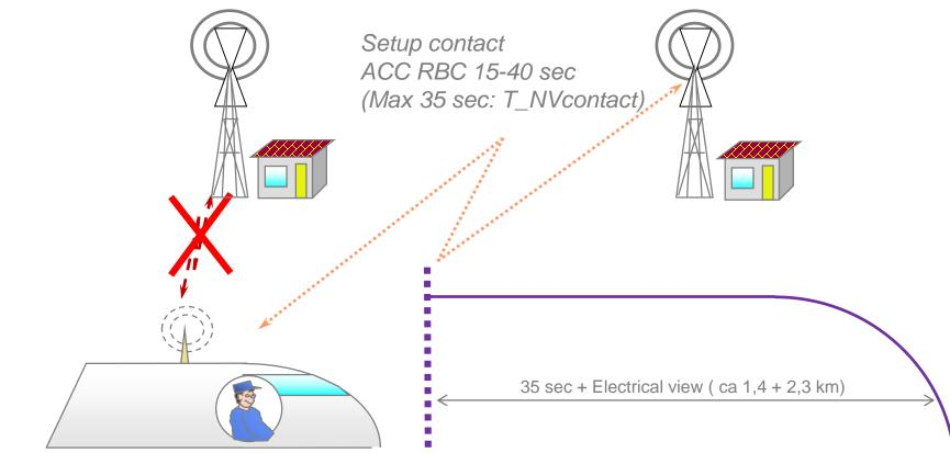
For a train with one modem or which has received a late RBC transition order the connection to the ACC RBC is established after the RBC-RBC transition. This takes nominally up to 40 sec. During this time no MA extensions are received. This has an performance impact and not also no CES or SMA can be received.
