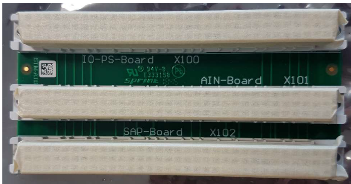
Definition, STMA-74579 - Figure: Analog Input Board front, coating example
