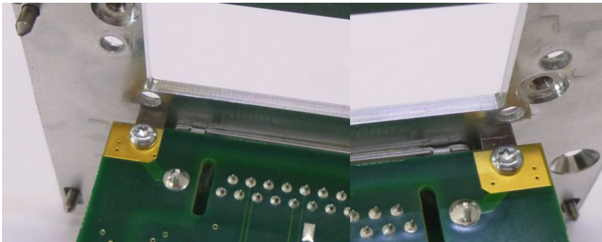
Definition, STMA-80457 - Figure: Mounting the AIN board to the front panel-2
